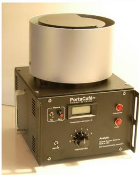
2. **A precision coffee sample roaster** that requires very little training to roast coffee repeatedly and consistently with a fixed temperature profile. It has an RTD bean temperature probe and an audible alarm controlled with an operator settable exit temperature; the two stage audible alarm alerts the
